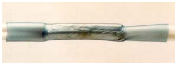
Acceptable: Solder has lost all appearance of ring shape. There is a definite fillet visible along the wire interface.
