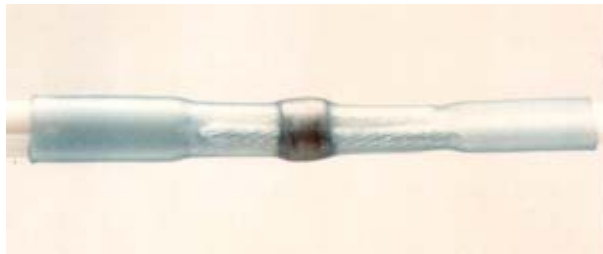
Unacceptable: Insufficient heat. Contour of solder perform is visible.
