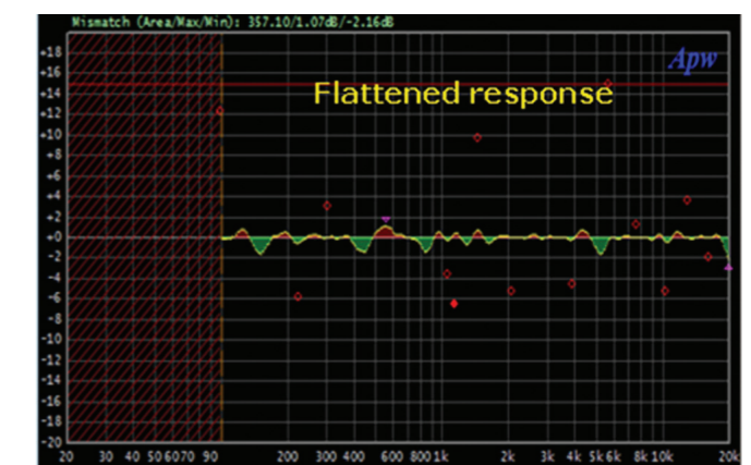
Speaker frequency response with STSpeakerTune™ compensation
