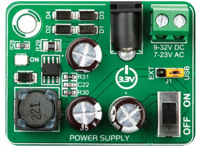
Figure 3-1: Power supply unit of mikromedia™ workStation v7
