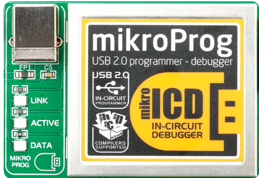
Figure 5-1: mikroProg™ is well protected under metal casing
