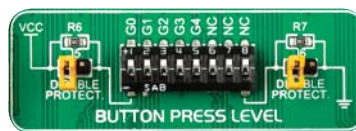
Figure 6-5: Button press level DIP switch (tri-state)
